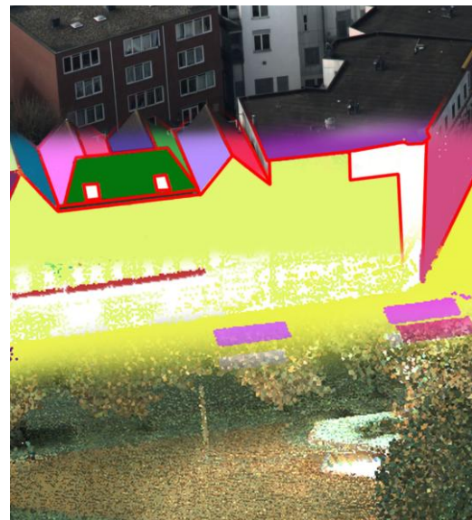
Obtaining the boundaries between surfaces, created from LiDAR data.
